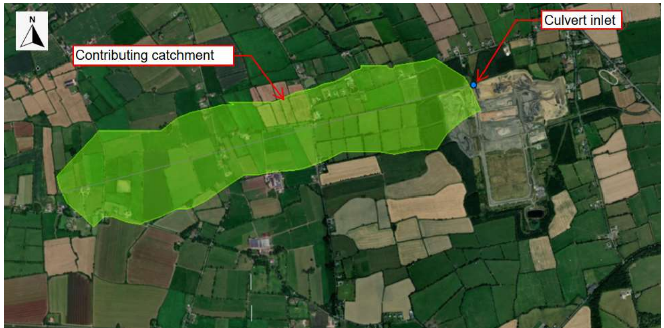
Figure 1 - Catchment boundary for the proposed culvert (OPW FSU, 2024)
